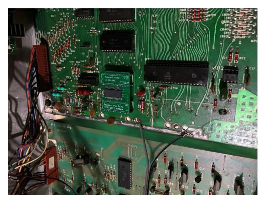
Here is the TPP-1011 NVRAM installed into both U13 and U9 sockets. A close inspection shows no pins were missed.
