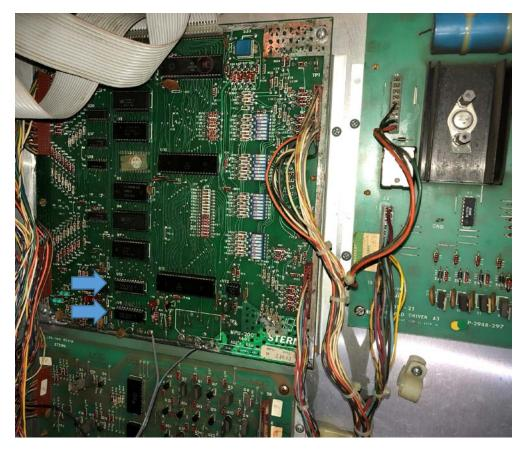
MPU-200 Board with original 5101 chips installed. The MPU-200 has these chips in sockets so removal is easy with a chip remover tool or a small screw driver.
