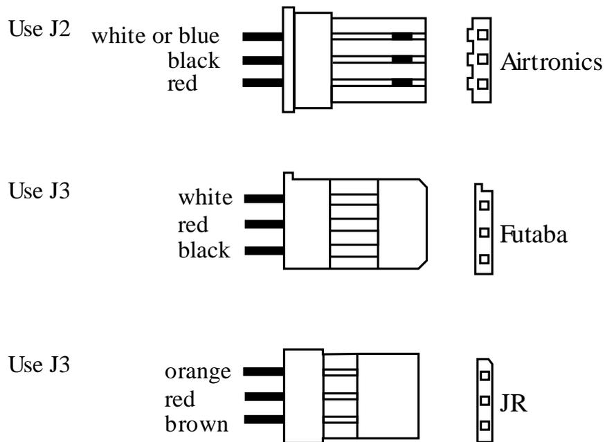
Please pay close attention to the colours of the servo wires. The servo must be plugged into the board with the correct orientation and into the correct plug (J2 or J3). The diagram above shows the commonly used wire colours for Airtronics, JR and Futaba servomotors. Noting the RED and BLACK or the RED and BROWN wires gives the best indication for how the plug must be inserted.
