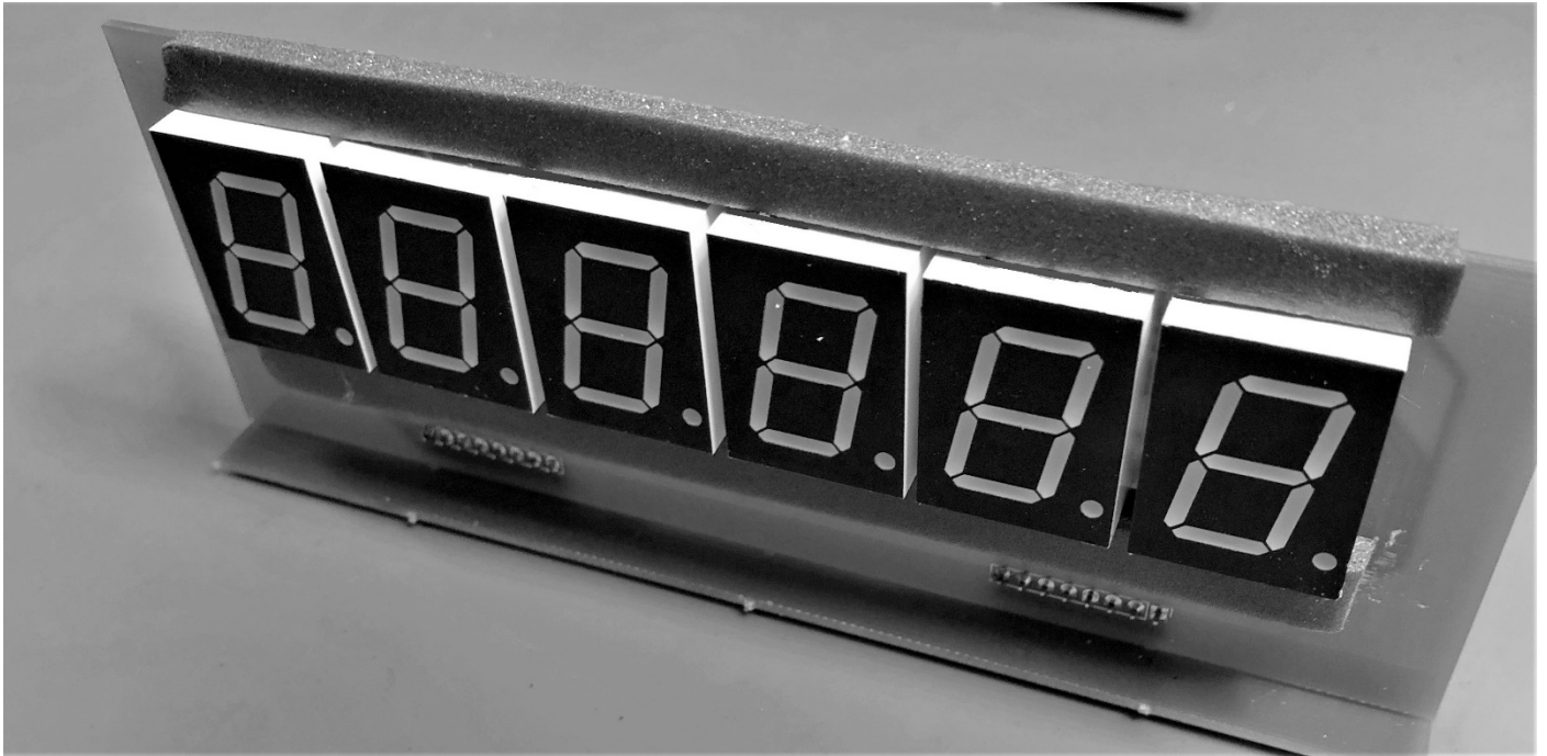
Photo 32: Foam tape installed on top and bottom of LEDs
