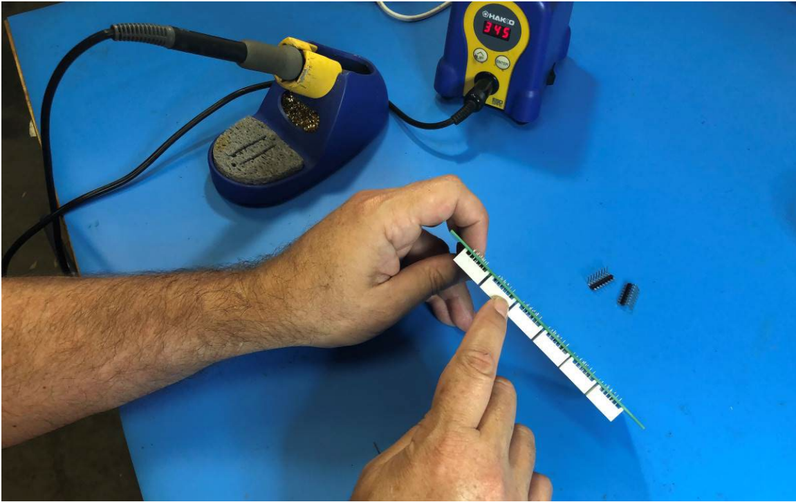
Photo 6: Check LEDs are positioned squarely and firmly against the PCB
