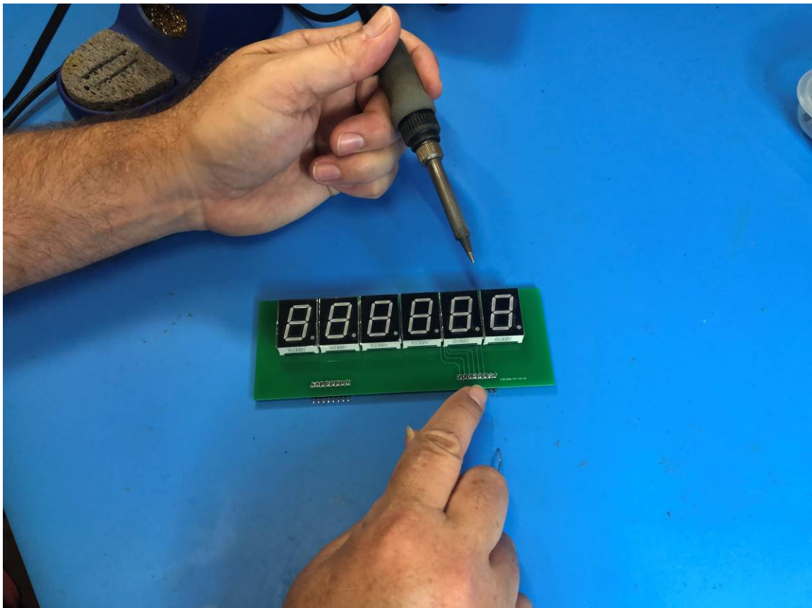
Photo 11: Flip the board over and check a good solder to the other side of the board. Add more solder if necessary.
