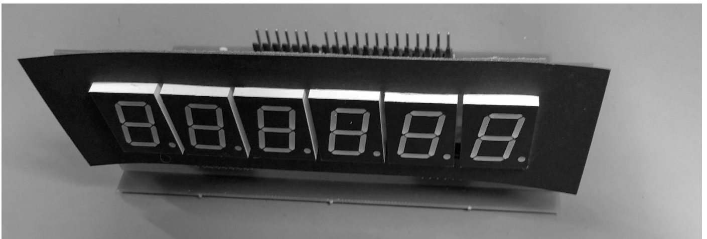
Photo 33: Card shroud installed on module. Ready for installation.
