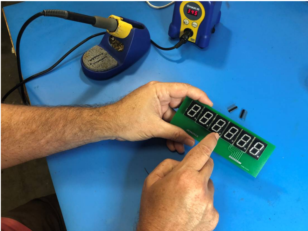
Photo 5: Re-Check the LED orientation
