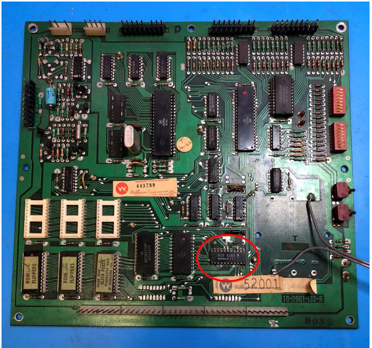
Williams System 6 board on the bench. The 5101 CMOS RAM is highlighted.
