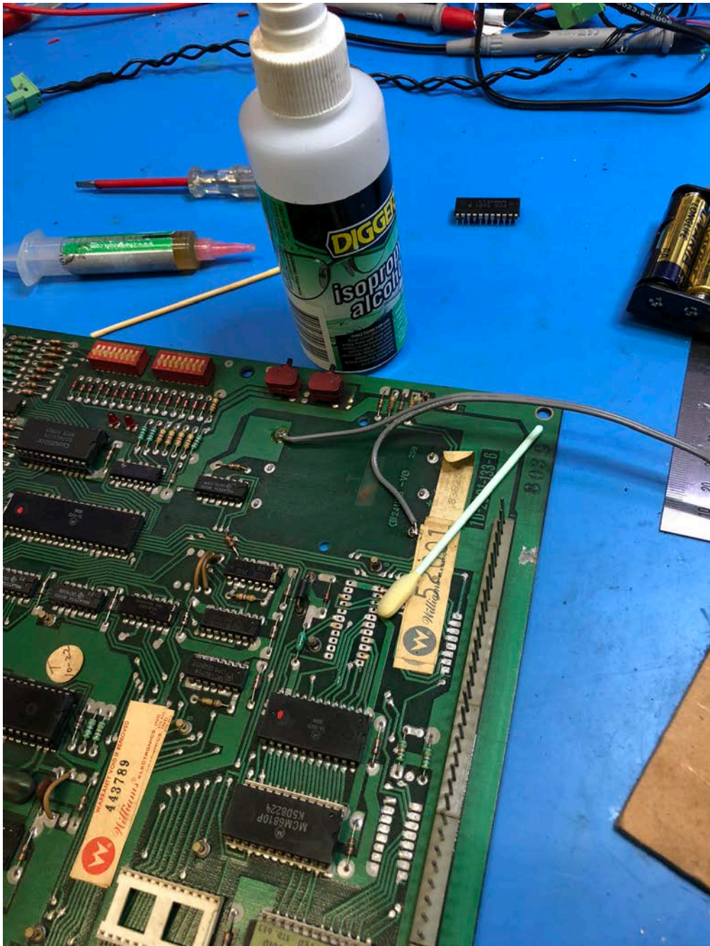
The 5101 has now been removed and isopropyl alcohol is used to clean the board.
