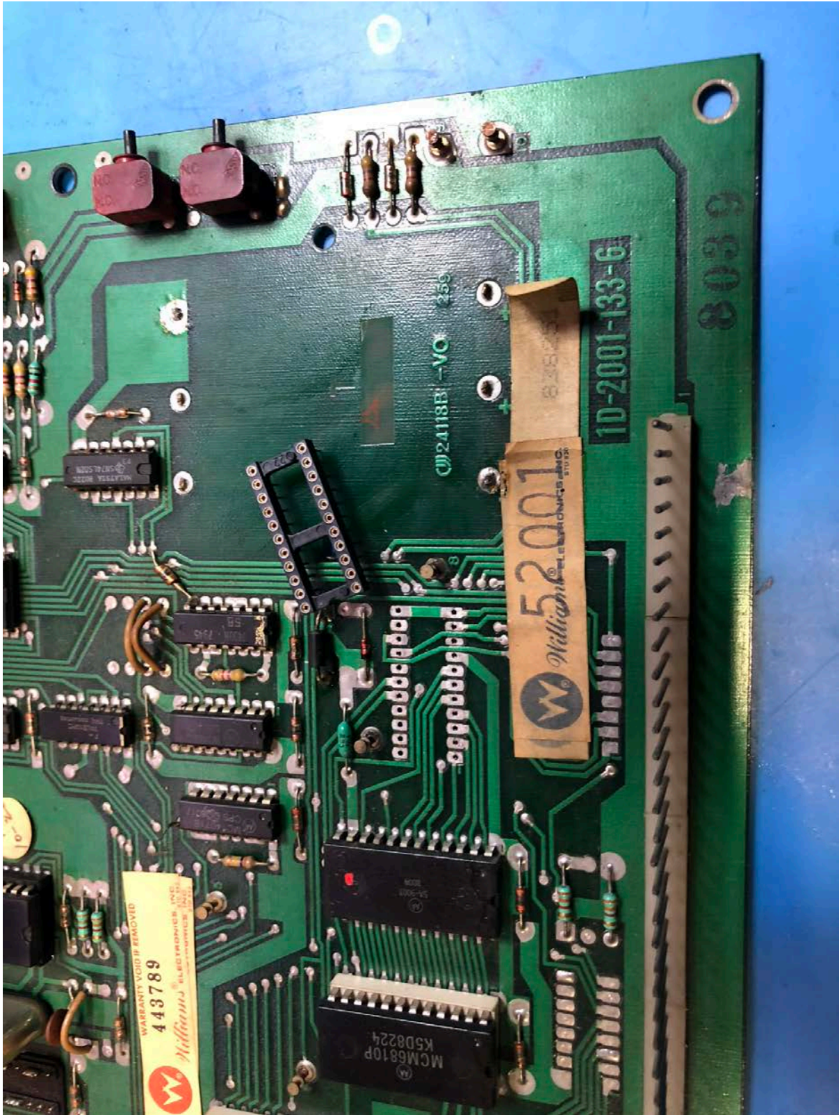
A turned pin socket is ready for installation.
