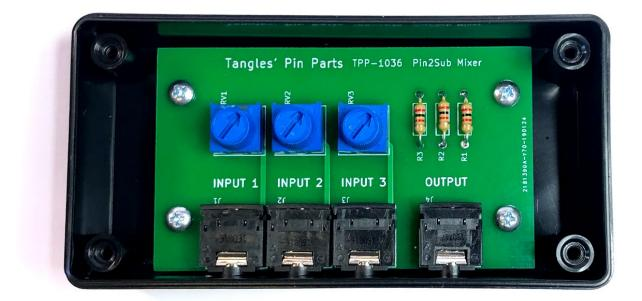
There are 3 level controls inside the Pin2Sub mixer if individual balance is required
