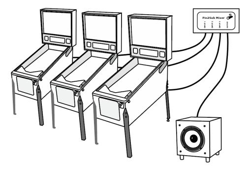
Connect up to three machines to a single Powered Sub
