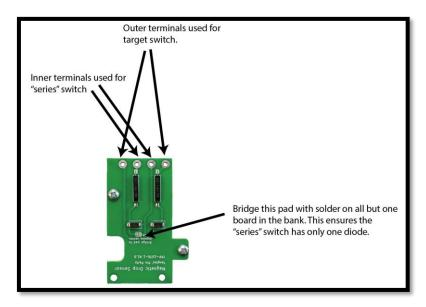
This picture shows a simplified wiring diagram of the "series" for Flash 3-Bank.
